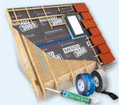
Fig. 45: Underlay membranes and accessories – associated products may be necessary to seal joints, tape over overlaps and seal nail penetrations; ideally, system components provided by the membrane manufacturer should be used.
