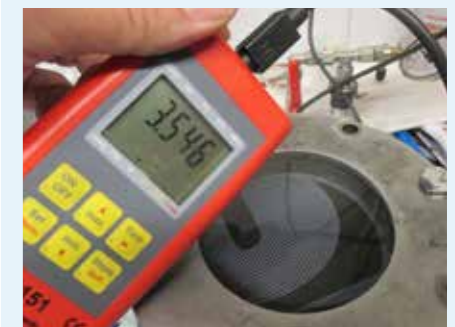
Fig. 23 a/b: Hydrostatic pressure test in the laboratory – overpressure is created using compressed air to simulate an artificial water column. Good-quality underlay membranes achieve values of over 2,500 mm.
