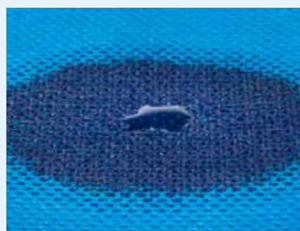
Fig. 25b: Water with reduced surface tension due to the presence of additional chemicals: no clear drop formation, the water tends to disperse and can pass through pores easier.
