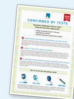
Fig. 39: The ageing resistance of airtightness adhesives can be tested in accordance with the DIN 4108-11 standard. Artificial ageing of 120 days corresponds to around 17 years. Ageing was extended to 700 days (corresponds to 100 years) for pro clima adhesion products.
