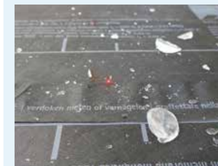
Fig. 33: SOLITEX underlay membranes installed over wood fibreboard panels remain undamaged even after repeated impacts with 50 mm hailstones.
